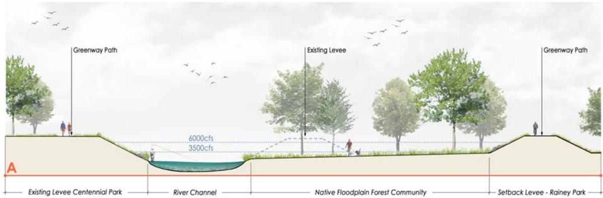
Figure 10. Rainey-Centennial Park Concept Showing Cross-Section
