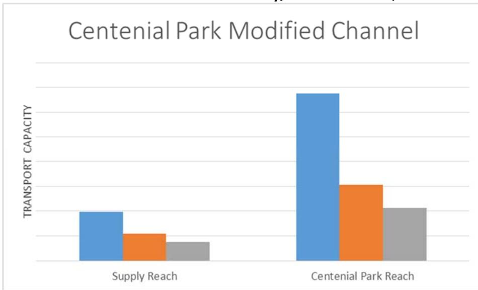
Supply reach is a river segment just upstream of the park, and represents the amount of sediment flowing into the park. Colors represent the transport equation used to calculate sediment loading. Blue uses Yang  $d_{50}$ , orange uses Laursen (Copeland), and gray uses Engelund-Hansen equations.
