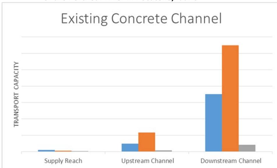
The channel is broken into two segments, an upstream and downstream reach. Supply reach is a river segment just upstream of the upstream reach of the concrete channel, and represents the amount of sediment flowing into this park. The upstream channel sediment was used as the sediment supply to the downstream reach. The colors represent the transport equation used to calculate sediment loading. Blue uses Yang  $d_{50}$ , orange uses Laursen (Copeland), and gray uses Engelund-Hansen equations.
