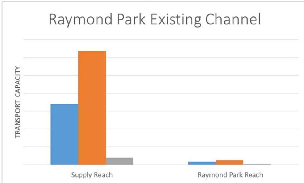
Supply reach is a river segment just upstream of the park, and represents the amount of sediment flowing into this park. The colors represent the transport equation used to calculate sediment loading. Blue uses Yang  $d_{50}$ , orange uses Laursen (Copeland), and gray uses Engelund-Hansen equations.
